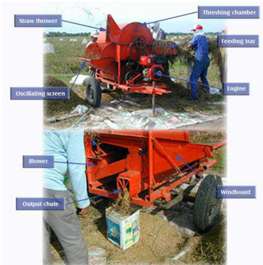
Figure 17: Components of an axial-flow, feed-in thresher with a cleaner
