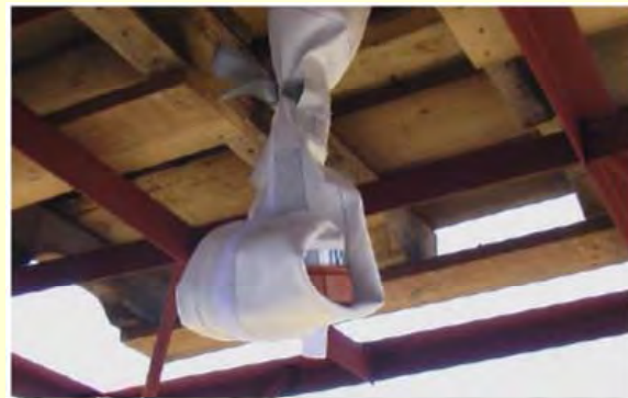
Undemeath the GrainSafe showing the tied downspout. Loosen the tie to start discharge of grains.
