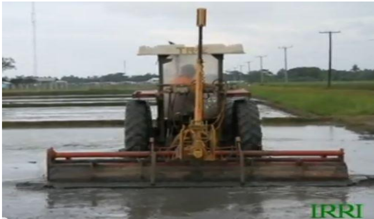
Laser Leveling with drag bucket
