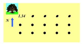
In the case of a land leveling exercise, where a cut/fill map is required, it is best to use the mean height of the field as a reference point. To determine the mean height of the field add together all of the measured points and divide by the number of measurements.
