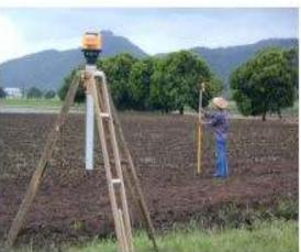
From the field diagram and knowing the mean height of the field, a strategy can then be determined to most effectively move soil from the high to low areas..
