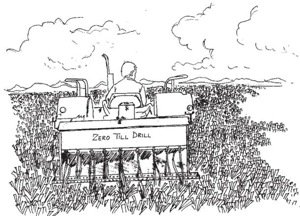
In the late 1980s, 34 zero-tillage trials were conducted on farmers' fields over three years in the rice-growing belt of the Pakistan Punjab. The implement used in these trials was a tractor-pulled seed and fertilizer drill with inverted-T openers. With this equipment, farmers could place the seed directly into the standing rice stubble without any land preparation.
