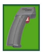
This non-contact thermometer can be used for monitoring grain temperature in post harvest processes like rice milling and drying.
