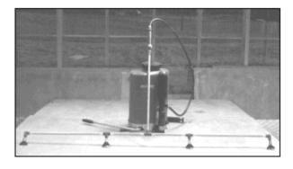
Flat fan nozzles are spaced on the boom so that the spray pattern of adjacent spray tips will overlap by thirty percent. Spacing will depend on boom height and the angle rating of the spray tips. Larger angle tips have a wider spray pattern and may be spaced further apart on the boom when the height remains constant.
