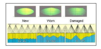
patterns should be checked at regular intervals and be replaced when worn and damaged.
