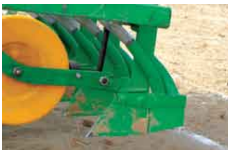
Seed drills with inverted-T tines are suitable for seeding into both tilled and nontilled soil.
