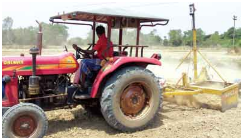
Land leveling using laser guidance
