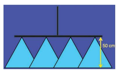
Boom height for desired spray pattern with slight overlap at ground level to avoid "misses"
