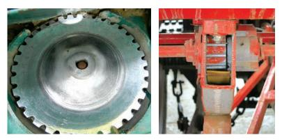
Inclined-plate (left) and fluted-roller (right) seed metering systems
