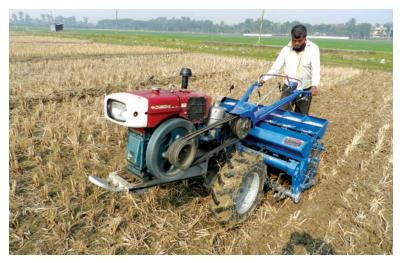
Crop being sown into rice stubble of the previous crop using a seedfertilizer drill with inclined-plate seeding mechanism, using strip tillage, powered by a 2-wheel tractor. Tillage and seeding are done in a single pass. Note the crop residues from the previous crop that remain on the surface of the soil after seeding (right).
