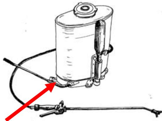
The spray tank contains liquid. There is an opening to put liquid in the sprayer. It has a built-in strainer and a cap.
