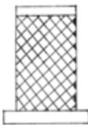
→ Strainer: Filters particles that can clog the nozzle
