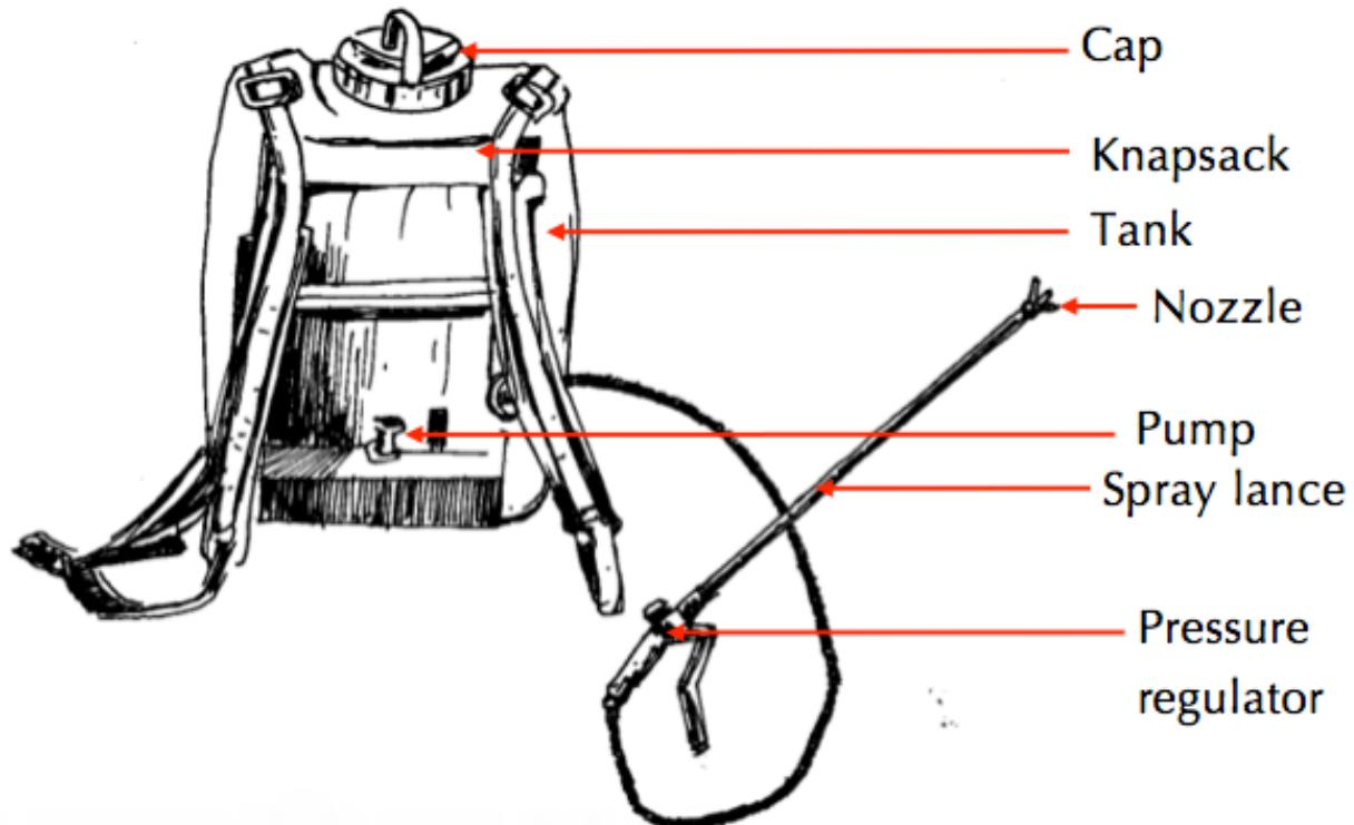
Pumps are an important part of the sprayer. They convert the water and herbicide into the spray mist.
