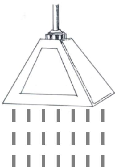
A hood for an even flat fan nozzle showing spray direction
