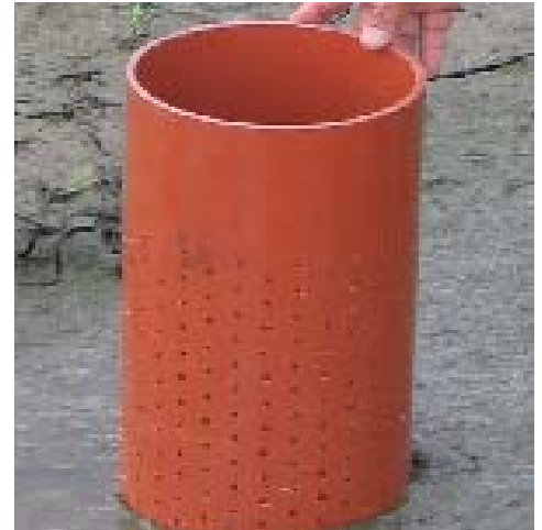
Field water tube from PVC Note the holes on all sides
