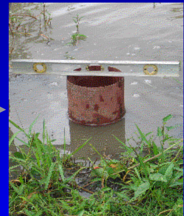
Check and level percolation tube
