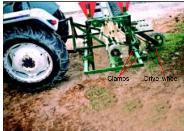
Fig. 14. Drive wheel attached on the rear side.
