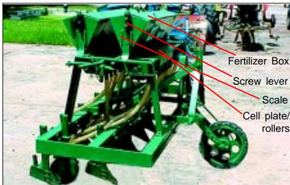
Fig. 31. Fertilizer metering device and its components.
