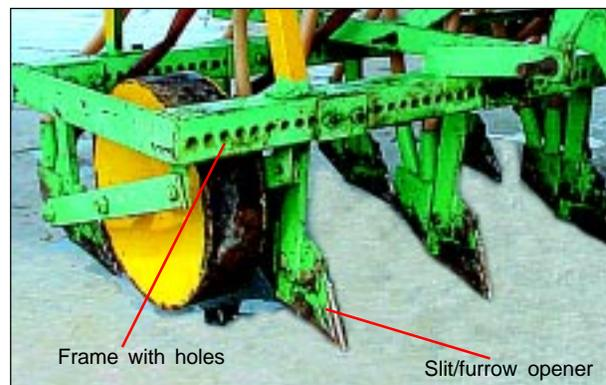
Fig. 4. Frame with holes, and slit/furrow openers.
