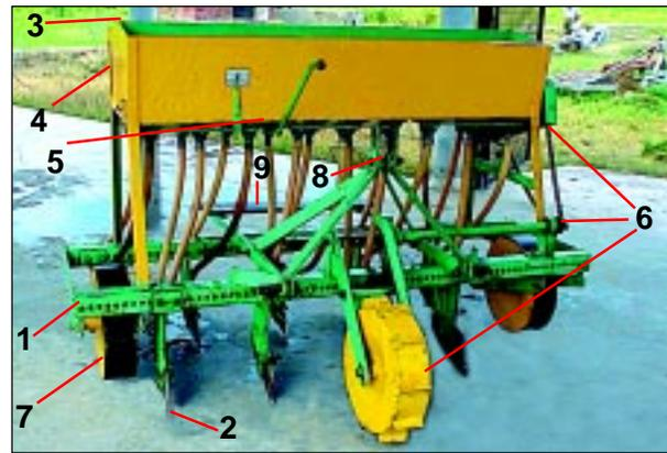
Fig. 3. Zero-till seed-cum-fertilizer drill and its major components.
