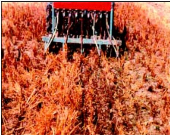
Fig. 19. Sowing of wheat with zero-till seed-cum-fertilizer drill in standing stubbles of paddy without burning.
