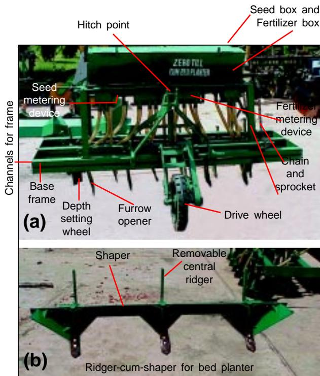
Fig. 20. Zero-till drill-cum-bed planter and its major components.
