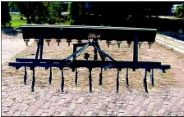
Fig. 2. Rabi seed-drill commonly used by farmers for conventional sowing.
