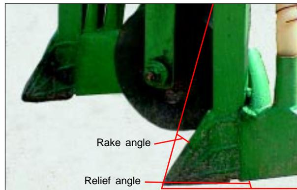
Fig. 22. Rake angle and relief angle of the furrow opener.
