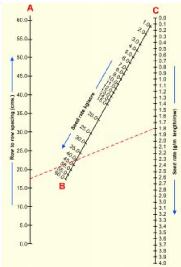
Fig. 10. Nomograph for seed-drill calibration.
