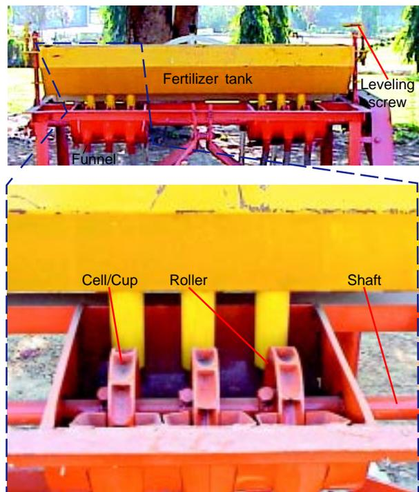
Fig. 12. Rotating cup/cell type fertilizer meter
