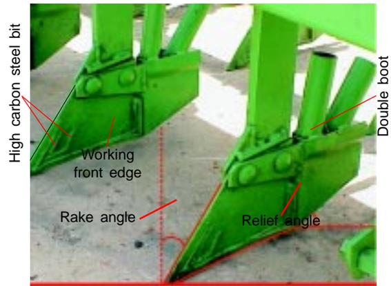
Fig. 7. Rake angle and relief angle of the furrow opener.
