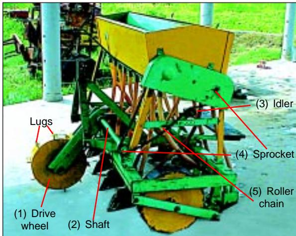
Fig. 13. Power transmission unit and its main components.
