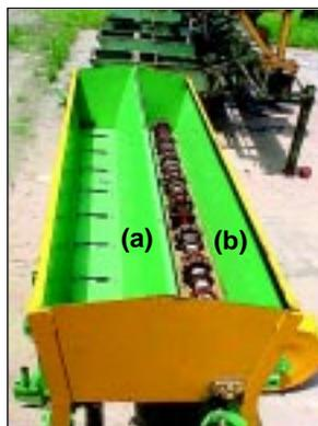
Fig. 8. Inner view of (a) Seed, and (b) Fertilizer boxes.
