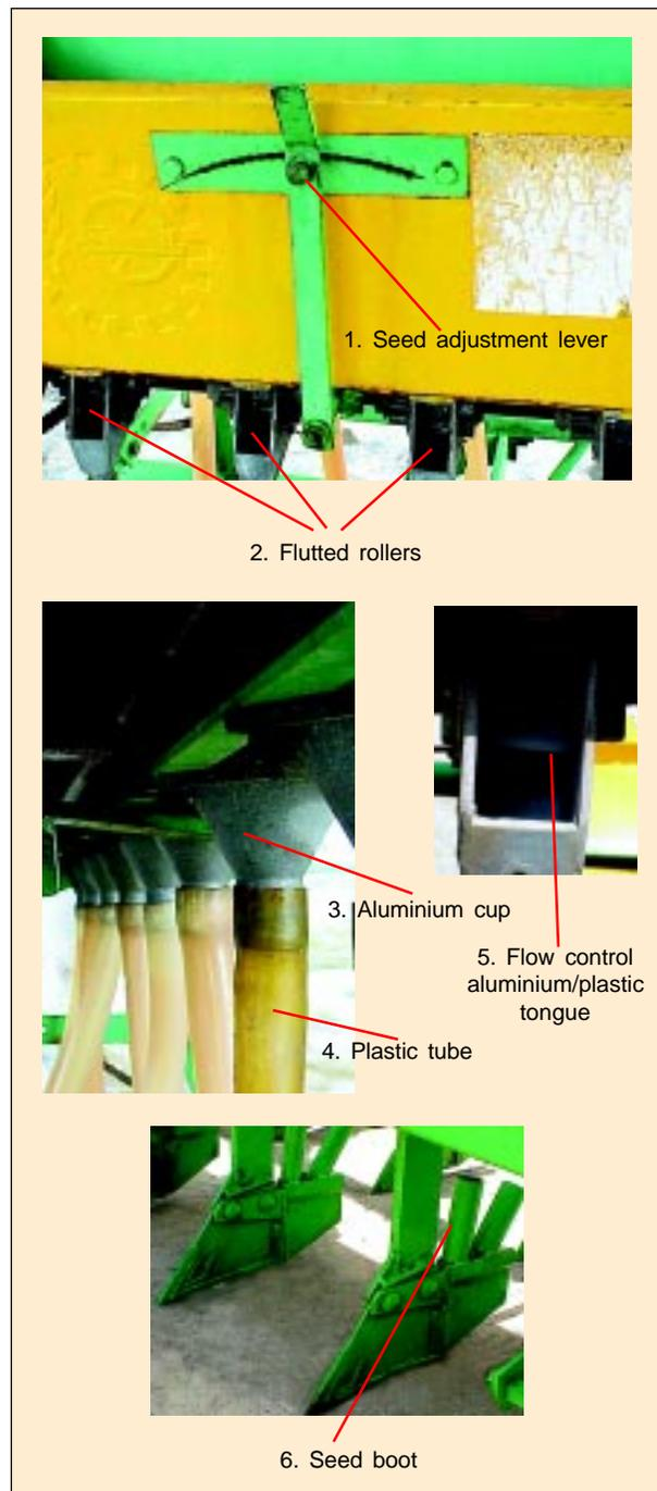
Fig. 9. Seed metering device and its components.
