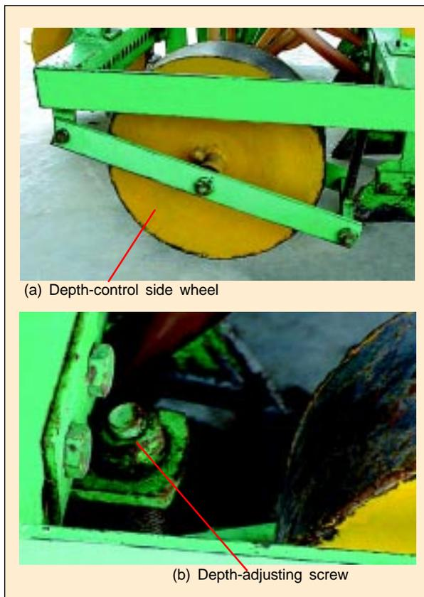
Fig 15. Depth-control side wheel (a) and depth-adjusting screw (b).
