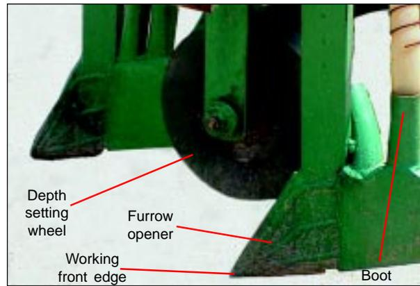
Fig. 21. Furrow openers of the zero-till drill-cum-bed planter.
