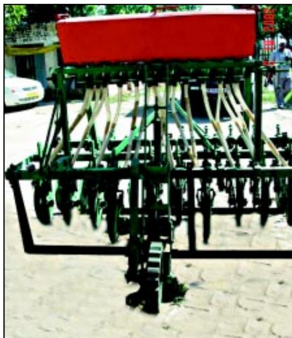
Fig. 1. Zero-till seed-cum-fertilizer drill — an improved version with disc openers under field testing.
