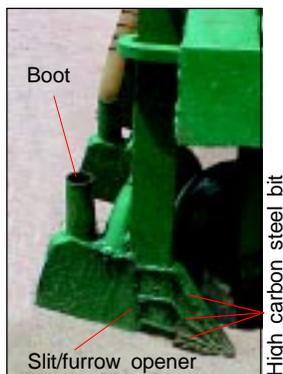
Fig. 6. Slit/furrow opener and the boot.
