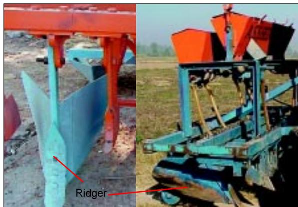
Fig. 24. Ridger of the zero till drill-cum-bed former.
