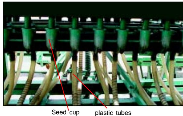
Fig. 28. Seed cup with plastic tubes.
