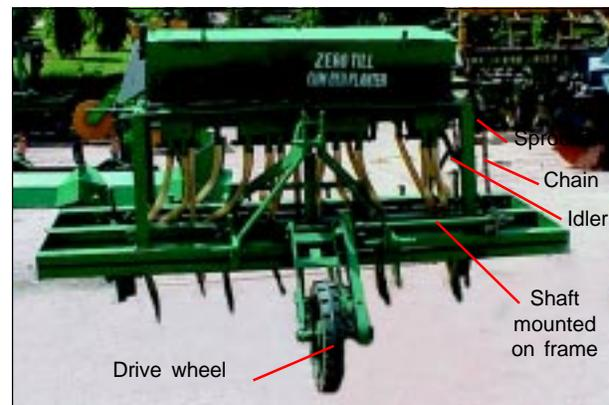
Fig. 32. Power transmission unit and its components.
