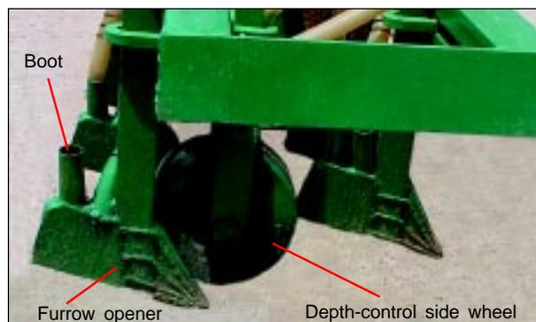
Fig. 38. Depth-control side wheel.
