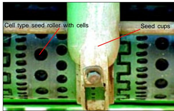
Fig. 27. Cell type roller and seed cup.
