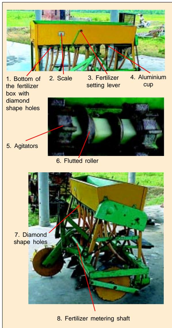
Fig.11. Fertilizer metering device and its components.
