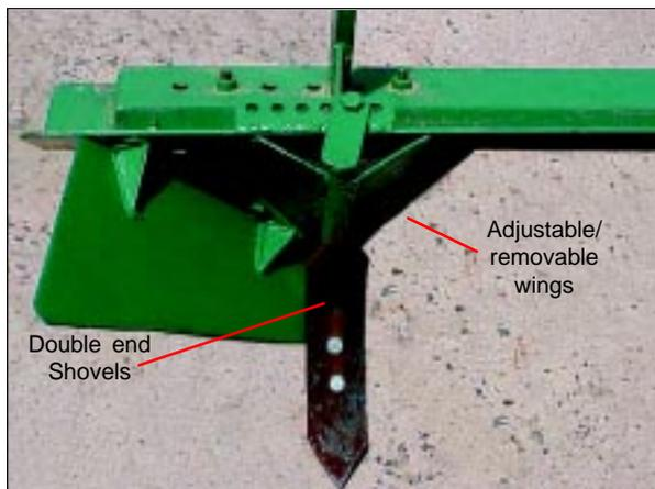
Fig. 23. Ridger, bed-cum-furrow shaper fitted with double end shovel
