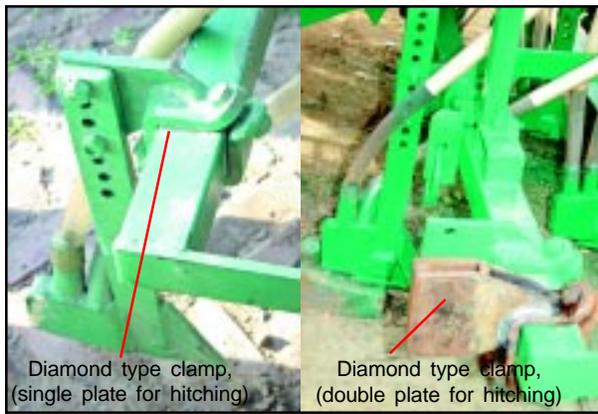
Fig. 5. Diamond/box type fastening clamps
