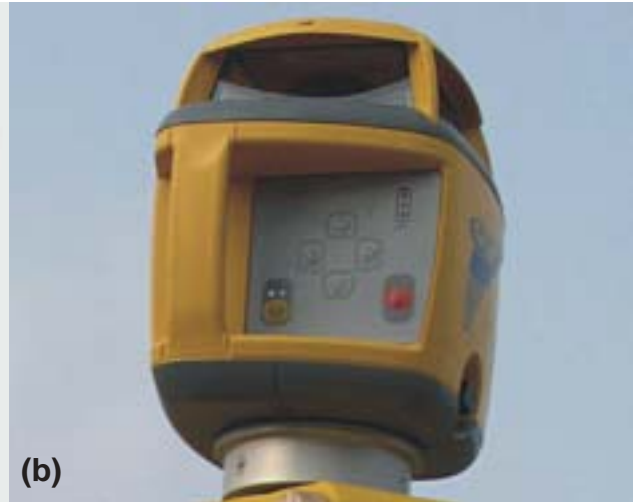
Figure 17. (a) A laser transmitter mounted on a tripod allows laser beam to sweep over the field (b) A close-up view of a laser transmitter
