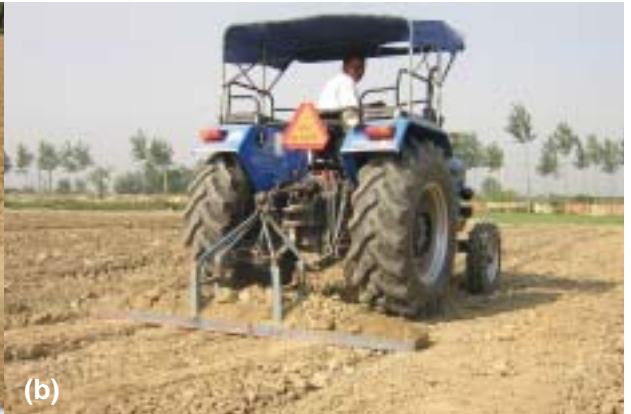
Figure 3. (a) Traditional method of land leveling using animal-drawn wooden log. (b) Mechanised land leveling using tractor-drawn planker
